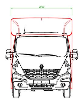
DEFLECTOR AND SIDEWINGS DRAWING CAN BE USED ON VAUXHALL MOVANO CAD DRAWINGS.
