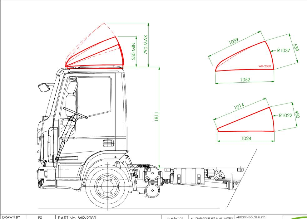
DRAWN BY PS PART NO. WR-2080 Issue No: 01 ALL DIMENSIONS ARE IN MILLIMETRES
