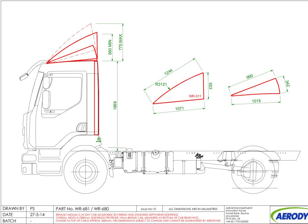
RENAULT MIDLUM 2.1M DAY CAB ADJUSTABLE 3D FAIRING AND STANDARD DEPTH REAR SIDEWINGS OVERALL WIDTH IS 2380mm. SIDEWINGS PROTRUDE 10mm BEHIND CAB, MEASURED AT BOTTOM OF CAB REAR FACE.
