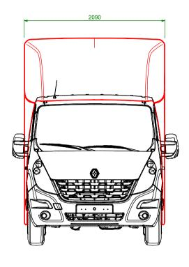
DEFLECTOR AND SIDEWINGS DRAWING CAN BE USED ON VAUXHALL MOVANO CAD DRAWINGS.
